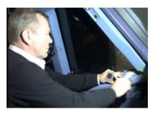
2) Using your other hand, lift the lower edge of the mount up and away from the window shroud.
