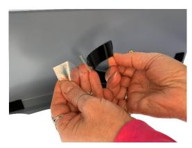
5) Measure the distance of the inboard channel which is free of any existing Velcro. Trim the new Velcro to fit between the existing Velcro. Do not allow any overlap onto existing material. This distance is approximately 9.75in / 245mm, but may vary.
