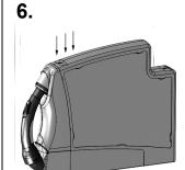
Install the Vroom in the mounting bracket by pushing it into place as shown. It will snap in place when installed correctly.
