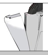
Before installing, remove bracket from the bottom of the Vroom by inserting a flat blade screwdriver into the release tabs located on each side of the mounting bracket as shown.
