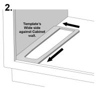
Locate cardboard template inside the cabinet. Place template's wide side against cabinet wall.
