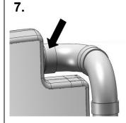
Connect the vacuum tubing to the Vroom's connector on the back as shown. Do NOT glue, press fit only for service reasons.
