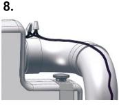
Connect the low voltage wires on the back of the unit.
