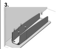
Place mounting bracket in template. Secure with 5 screws as shown.
