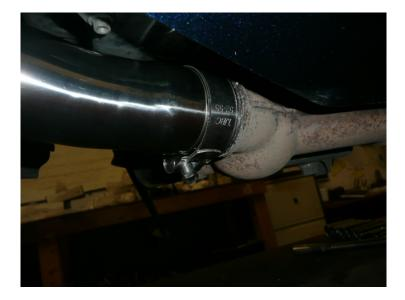
*Insert silencer with clamp on to link pipe. Now fit strap onto silencer and to frame.*
