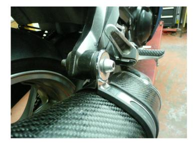
Repeat on the other side. Rotate link pipes to obtain alignment and clearance. Fully tighten all clamps and fasteners. Start engine and check for leaks. After your first ride out, check all fasteners for tightness, especially the baffle bolts.
