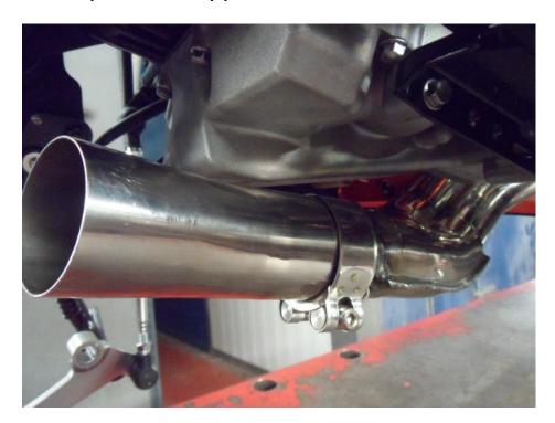
• Fit the silencer with clamp on to the link pipe and fit the strap around the silencer and to the frame.
