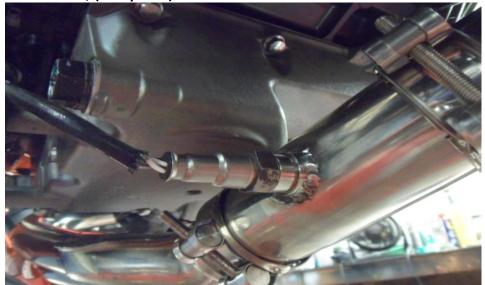
• Starting from the front, working rearwards tighten all clamps and fasteners, double checking clearances to the plastics.
