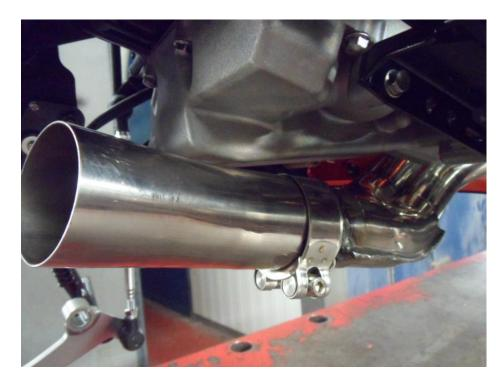
• Fit the clamp and insert the pipe on to the collector.
