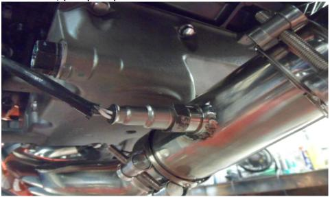
• Starting from the front, working rearwards tighten all clamps and fasteners, double checking clearances to the plastics.
