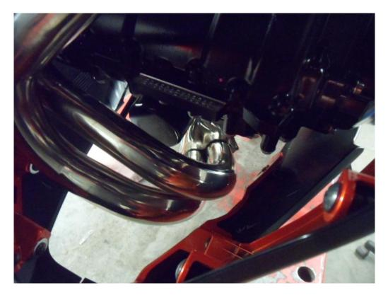
• Fit the carbon gasket on to the collector.
