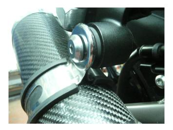
HINT. Use soapy water on rubber strap to ease adjustment. Rotate link pipes to obtain true alignment and clearance. When you are happy, starting from the front, tighten all clamps and fasteners. Clean off any soap, excess silicon and finger marks. Start engine and check for leaks. Replace panels, seats etc. After your first ride out, check all fasteners for tightness, especially the baffle bolts.
