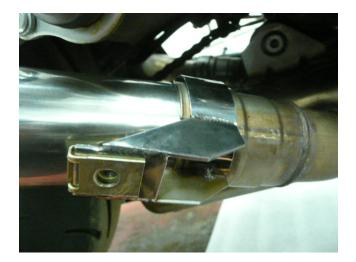
Nip up bolt not too tight for now, just to support pipe. Smear a light coating of sealant inside silencer and fit with clamp on to link pipe. Now fit strap onto silencer and to frame.
