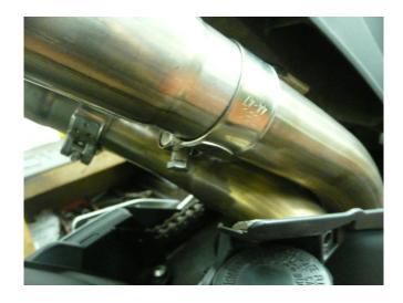
Nip up bolt not too tight for now, just to support it. Smear a light coating of sealant inside silencer and fit with clamp on to link pipe. Now fit strap onto silencer and to frame.
