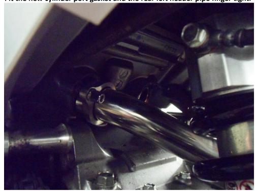
• Fit the new cylinder port gasket and the rear right header pipe finger tight.
