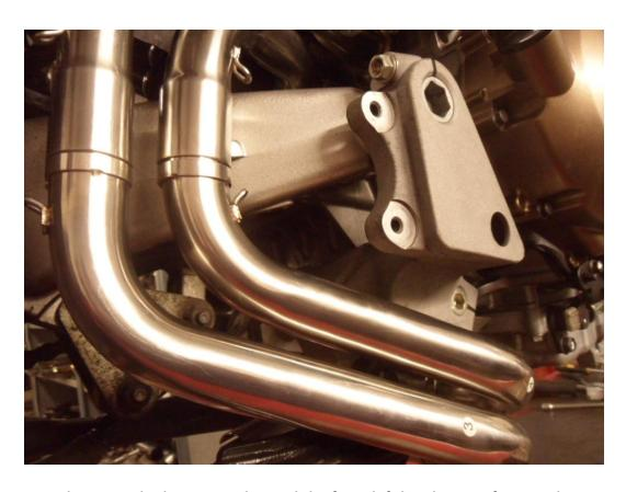
• Fit the new cylinder port gasket and the front left header pipe finger tight.
