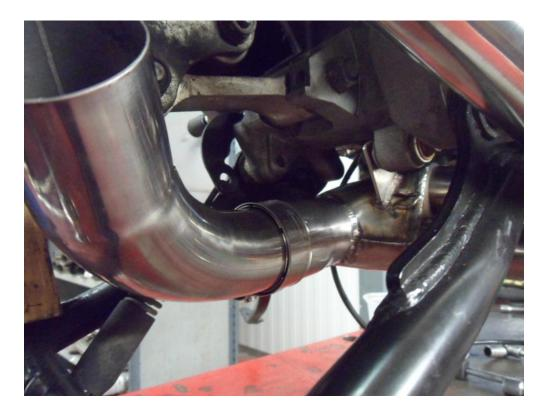
• Fit the link pipe and the silencer and then fit the strap around the silencer and to the frame.
