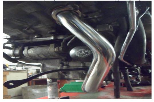
• Fit the new cylinder port gasket and the front right header pipe finger tight.
