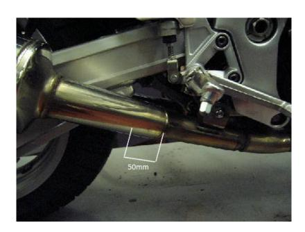
The Delkevic link pipe and silencer can now be fitted to the original downpipe (use a sealant on joints if required).
