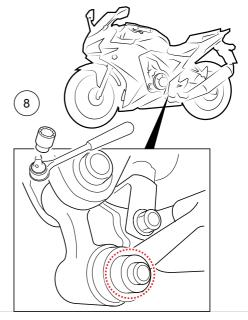
Remove the bottom shock mount by loosen bolt and nut with 14 mm and 17 mm socket.
