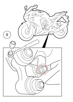
Remove the top shock mount, by loosen bolt and nut with 14 mm and 17 mm socket.
