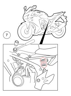
8 Remove rear pull rod, by loosen bolt and nut with14 mm and 17 mm socket.
