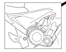
2 Loosen the screw with a 5mm Allen key.
