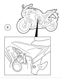
7Loosen the bolt that hold the regulator with10mm socket, move it a little to the side.
