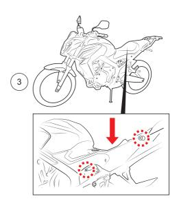
**4**Remove the outside front fairing on both sides by loosening the three screws.
