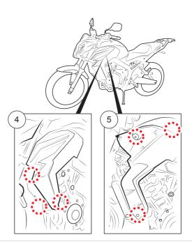
6 Loosen the bolt and lift the fuel tank up in the order to access upper bolt
