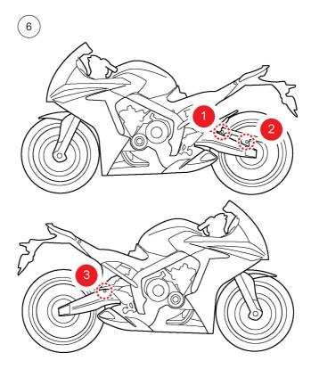
Remove the standard shock absorber by loosening the upper (1) and the lower (2) bolts.
