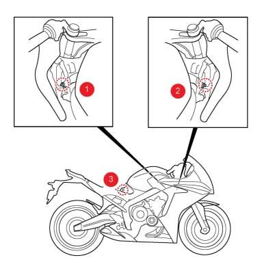
**6** Remove the chain guard by loosening the three bolts (1)(2)(3).
