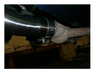
Smear a light coating of sealant inside silencer and fit with clamp on to link pipe. Now fit strap onto silencer and to frame.
