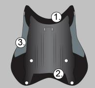
As a first step, pull the lining towards the opposite side of the saddle and nail it with the staple gun the fixing it with 2/3 staples.(4)
