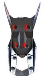
7. Assemble cover plate to the main bracket (see picture below). Feed the indicator wires through the slot before securing the bracket into position using 2 x M4 x 10mm countersunk screws.
