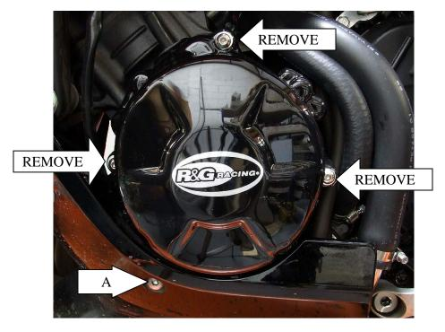
In this kit there should be 1 x Engine Case Cover (ECC0021R) 3 x M6x40mm Long Cap Head Bolts
