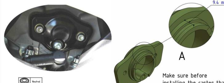
Make sure before installing the carter that the size shown in the figure (A) must be identical to the original case.
