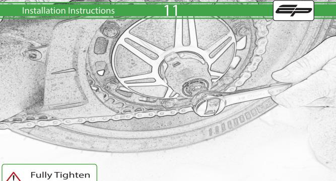
Fully Tighten 8Nm
