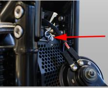
2. Fit new bracket supplied using the four original bolts shown in picture.
