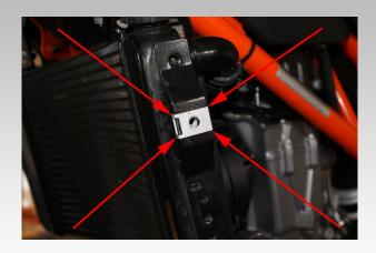
4. fit the radiator guard as shown in the picture. Ensure the radiator guard tabs are positioned inside the radiator bracket.
