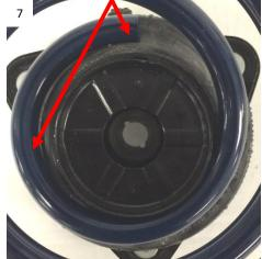
555-8214 and 555-8222 kits must trim the factory bump stops for proper suspension travel. The Front bump stops must be trimmed 1" and the rears trimmed 1.25" inches.
