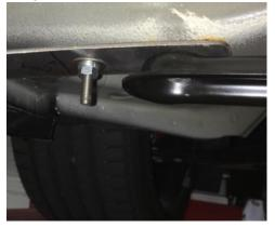
Figure 5: Steeda jacking rail front bracket
