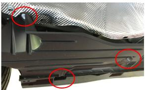
Figure 1: Rear plastic cover hardware
