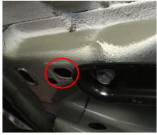
Figure 4: Slotted hole for offset stud
