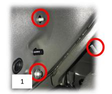
Figure 1: Factory taillight nuts
