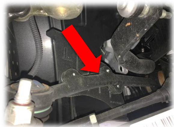
Figure 2: Factory tension link
