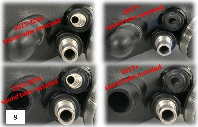
Figure 9: Steeda intake tube hose connection configurations
