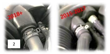
Figure 2: Hoses connected to factory intake tube
