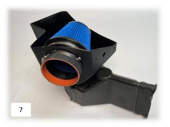
Figure 7: Steeda airbox assembly
