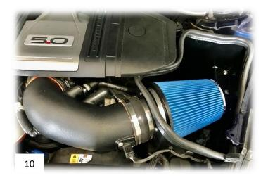
Figure 10: Steeda air intake system installed
