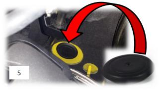
Figure 5: Sound tube plug installed
