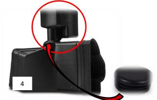
Figure 4: Factory resonator on inlet duct and Steeda plug
