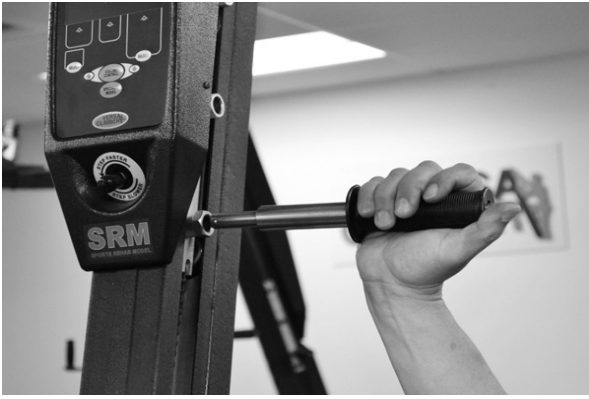
Install straight handgrips by depressing pin with thumb and insert.
