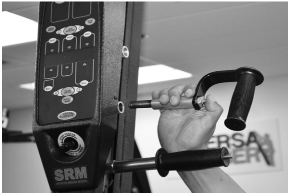
Install running handgrips by depressing pin with thumb and insert.
