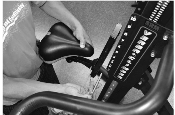
Apply seat bracket to post in desired position. Insert pull pin through frame and seat bracket.
