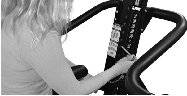
Mounting seat bracket assembly to post.
