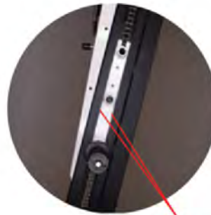
There are 2 lube port holes, one on either side of the bar assembly. Both ports require lubricant.
