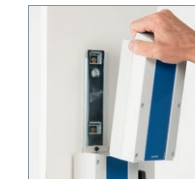
Spare battery on the wall charging station
