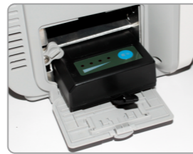
Dual Li-ion batteries, up to 10 hours of continuous work
