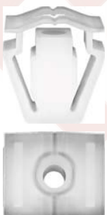
22308 (Audi: 8K0-821-213A) Natural Nylon Bumper & Side Air Baffle Retaining Clip Head Size: 15.3mm x 18.3mm Overall Height: 20mm Audi A4, A5, A6, Q3, Q5, RS7, S4, S5, S6, S7 & SQ5 2015 - On
