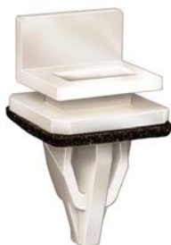
17096 (91513-SM4-000) Nylon Rocker Panel Moulding Clip Width: 20mm Length: 20mm Fits into 12mm Hole Accord 1991 - On UNIT PACKAGE: 10
