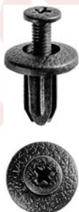
19142 (91550-SH3-003) Black Nylon Pillar Garnish, Side and Trunk Lining Push-Type Retainer Head Diameter: 15mm Stem Length: 13mm Fits into 7mm Square Hole Civic, Accord Wagon & Del Sol 1993-On
