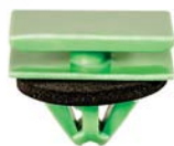
21504 (GM: 10445899) Black Nylon Door Moulding Clip Top Head Size: 14mm x 20mm Bottom Head Size: 15.5mm x 20mm Stem Length: 14mm Fits into 9mm Hole GM SUV's 1997 - On
