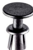
20666 (22677979, 22677980) Gray Nylon Door Trim Push-Type Retainer Head Diameter: 12mm Stem Length: 14mm (Excluding the Pin) Fits into 6mm Hole Chevrolet Malibu 2004 - On
