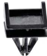
21504 (GM: 10445899) Black Nylon Door Moulding Clip Top Head Size: 14mm x 20mm Bottom Head Size: 15.5mm x 20mm Stem Length: 14mm Fits into 9mm Hole GM SUV's 1997 - On
