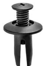
21089 (W710250-S300) Black Nylon Rear Bumper Push-Type Retainer Head Diameter: 18mm Stem Length: 18mm Fits into 8mm Hole Ford Edge 2007 - On
