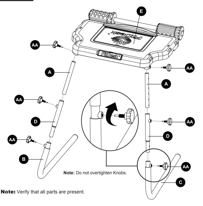
**Step 1:** Attach the Desktop **(E)** and the Inner Tube **(A)** on both the left and right sides. Tighten using one of the six Knobs **(AA)**. **(Note:** All Knobs are the same and can be used in any of the legs.)
