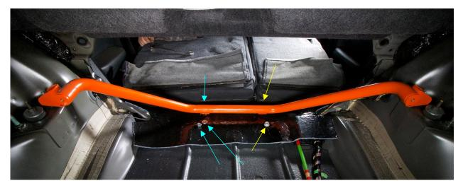
12. ADD CROSS BAR AND INSERT ONE BOLT ON EACH SIDE TO HOLD TO MAIN STRUT BAR
