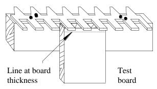
Move template with reference to mounting block
