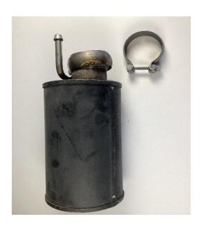
Longer Pipe Is Drivers Side And Shorter Side Is Passenger Cut as close to the resonator as possible
