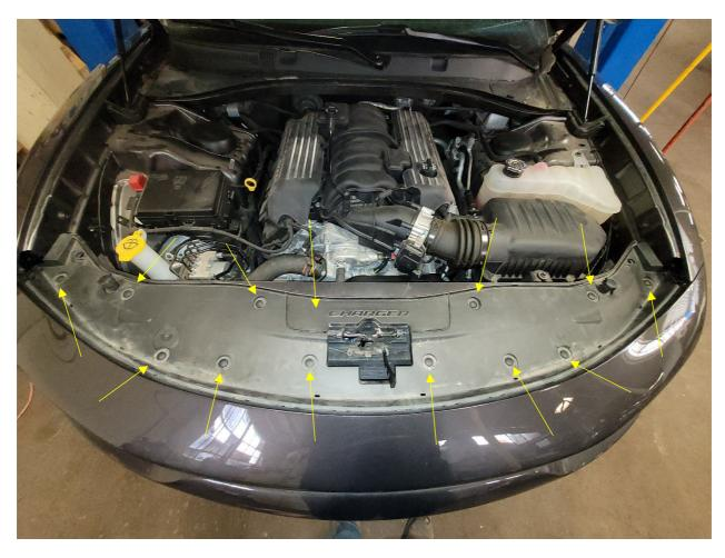
5. LOCATE AND REMOVE 2 10MM BOLTS HOLDING BUMPER TO FENDER
