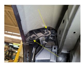
11. SLIDE UNDER THE FRONT OF THE CAR, LOCATE AND REMOVE 4 10MM BOLTS AND 3 OR 5 PLASTIC PUSH CLIPS
