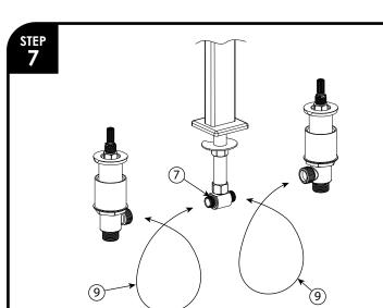
Connect stainless steel flex lines (9) from valve outlets to spout tee (7). Flex lines should be looped as shown in diagram. FLEX LINES MUST NOT BE KINKED. Adjust valves and or spout tee to eliminate any kinking in the flex lines. Install escutcheons onto the valves and hand tighten. DO NOT OVER-TIGHTEN. Install handles onto valve stems.
