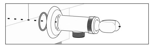
Slide Flange against the wall. **NOTE:** the hook is tapered to accept the cone fitting of hand shower hose. If the hose will not slide into the hook, rotate the hook assembly 180°.
