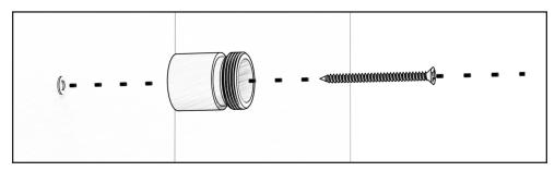
Slide flange and o-ring onto the bracket body.
