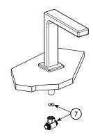
Install spout tee assembly (7) as shown in diagram.
