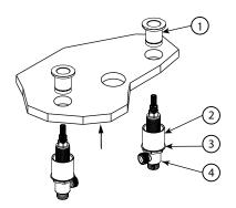
Remove top fastening nut and washer (1) from the lavatory valve. (NOTE A: All lever handle sets are supplied with one right-hand valve and one left-hand valve. Install valve with blue dot o the cold side. Insert valve from below through hole in lavatory or countertop.
