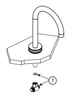
Install spout tee assembly (7) as shown in diagram.
