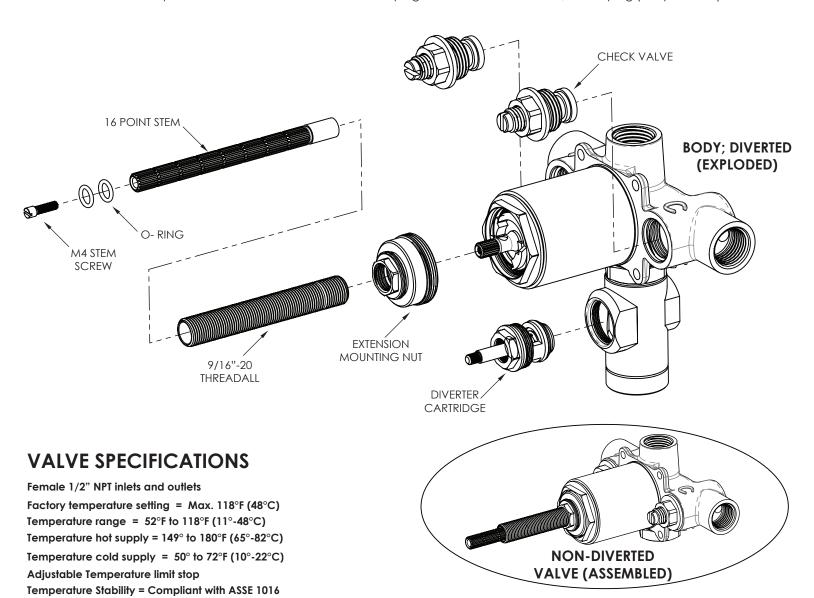
Recommended supply pressure = 20 to 80 psi (1,38-5,52 bar) Recommended hot water supply temperature = 120°F to 140°F (48°C-60°C)
