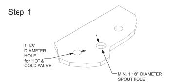
Should a counter top need to be drilled, please reference the diagram above.
