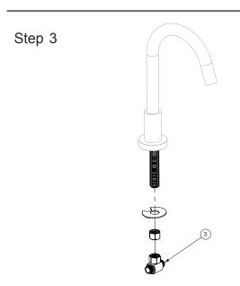
Install spout tee assembly (3) as shown in diagram.
