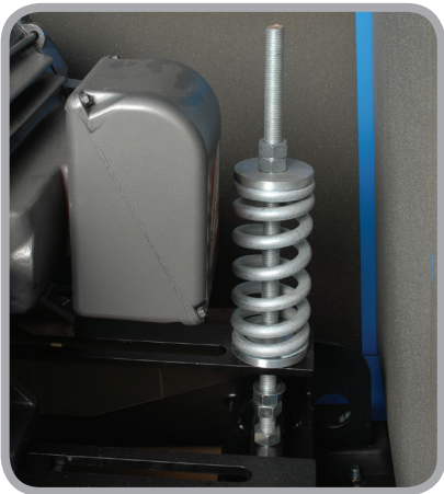
Automatic V-belt drive tensioning system
