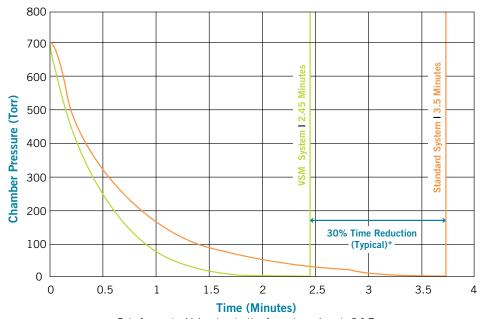
Data from actual laboratory testing from atmosphere to 0.1 Torr.
