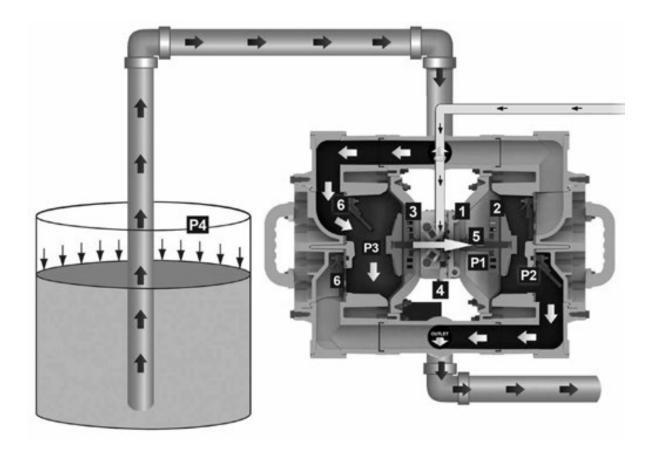
Air-Operated Double Diaphragm (AODD) pumps are powered by compressed air, natural gas or nitrogen.
