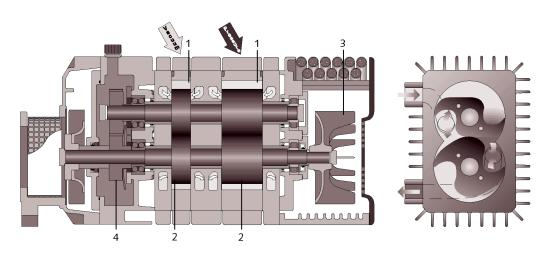
1. Compression chamber 2. Rotary claw 3. Fan 4. Gear
