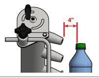
The pitch of the manifolds can be adjusted using the knob on the end of the manifold. The nozzles should be tilted about 10° down, to blow the water off and down the product.
