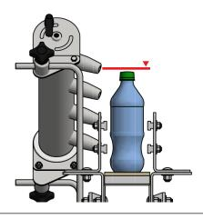
Using the knobs on the air knives, adjust the knives to be within 4" of the product being dried.
