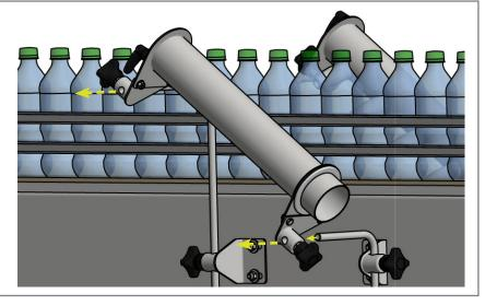
Adjust the height of the nozzle manifolds, by loosening the knob on the rod and sliding the rods up or down, so that the top nozzle is just above the top of the product, and the bottom nozzle is just below the bottom of the product on the conveyor, to ensure full drying coverage.
