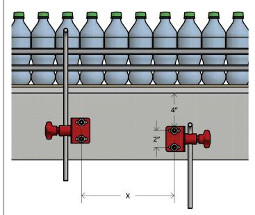
Where X = distance between rod mounting brackets, as shown in the table
