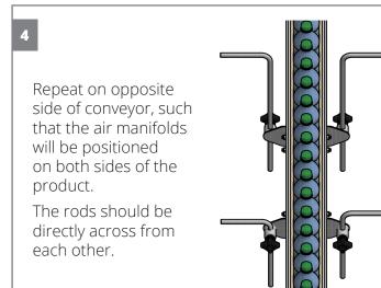
Install air manifolds by sliding the two rods through the two knobs on the air manifold brackets on either end of the manifold.
