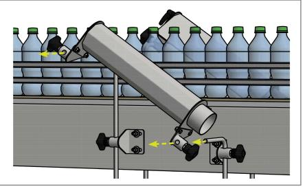
Adjust the height of the air knives, by loosening the knob on the rod and sliding the rods up or down, so that the top of the air knife is just above the top of the product, and the bottom is just below the bottom of the product on the conveyor, to ensure full drying coverage.
