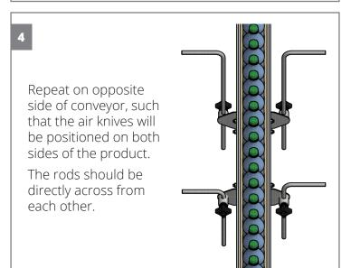
Install air knives by sliding the two rods through the two knobs on the air knife brackets on either end of the air knife.
