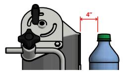
The pitch of the air knives can be adjusted using the knob on the end of the air knife. The air knife should be tilted about 10° down, to blow the water off and down the product.
