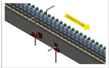
Using the knob, adjust the height of the upstream rod so that the top of the rod is at about the height of the product on the conveyor.
