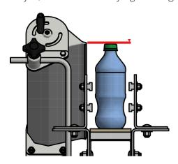
Using the knobs on the air knives, adjust the knives to be within 4" of the product being dried, preferably as close as possible.
