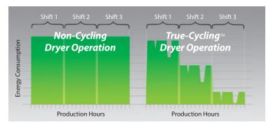
In applications with varying air usage and shift demands, and where there are daily and seasonal changes in ambient temperature, HeatSink™ True-Cycling™ operation provides a way for compressed air users to minimize energy cost associated with air treatment.
